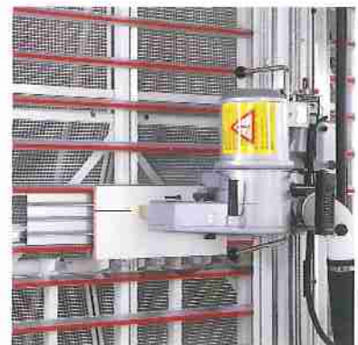
Cutting on the central support with the small workpiece support
