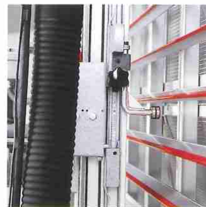
Strip cutting gauge for identical horizontal cuts
