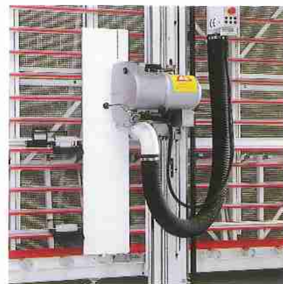
Vertical cutting with narrow pieces of panel using auxiliary stops
